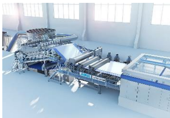
ANDRITZ wetlaid technology for glass fiber mats
